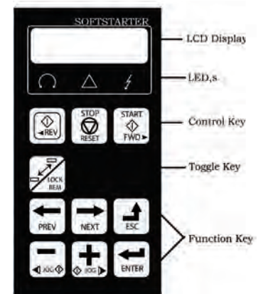
Fig. 7.30: Panel description of VFD
