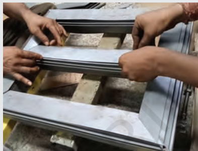
Fig. b: Assembling the number cores that are being cut
