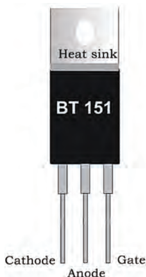
Fig. 7.31: Silicon control rectifier
