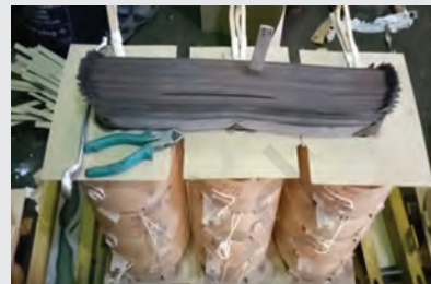
Fig. i: Insertion of I section in the core
