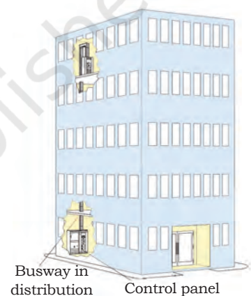
Fig. 1.41: Busway used in the distribution system
