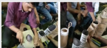
Fig. f: Insertion of insulation paper in the core of a three-phase transformer
