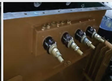
Fig. m: Fitting low voltage bushing on the transformer
