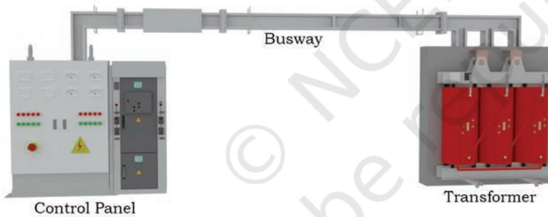
Fig. 2.6: A busway in a power distribution system
