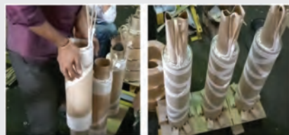
Fig. g: Insertion of a secondary coil in the core
