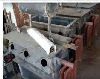
Fig. e: Making the main tank and the oil tank
